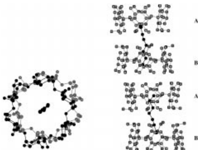
Figure 3. Description of the \alpha -(CD) 2 -C 4 H 9 NCS. 9 H 2 O complex. Left: View along the molecular axis of the \alpha -CD showing two \alpha -CDs containing one ITC. Right: View of two unit cells of the complex, illustrating the two orientations of the ITC molecules. Water molecules are not shown for the sake of clarity.
